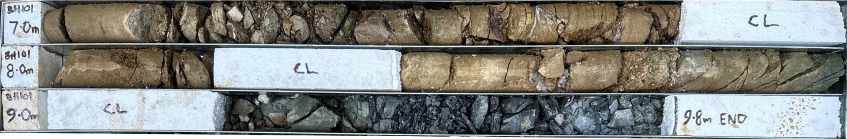
Core Recovery BH101 Start Core at 7.0m depth EOH at 9.8m Depth
