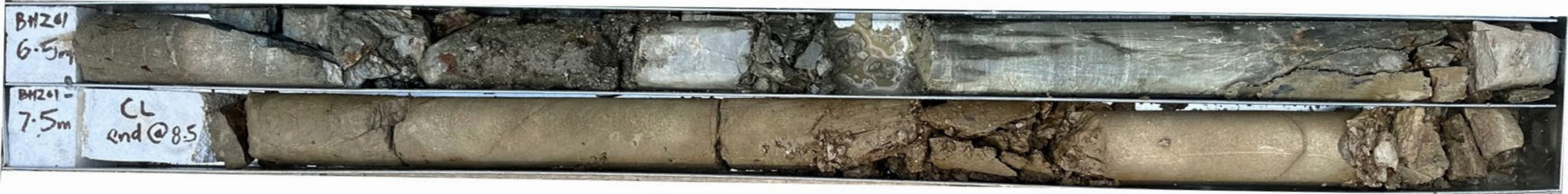
Core Recovery BH201 Start Core at 6.5m depth EOH at 8.5m Depth
